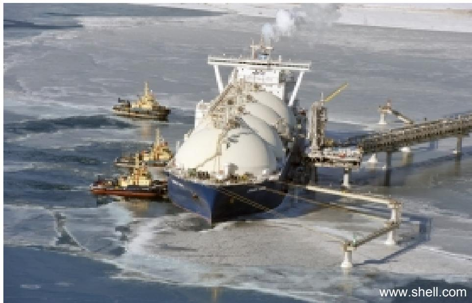
**Figure 52** LNG tanker approaching the jetty head with tug boat assistance in light ice conditions
