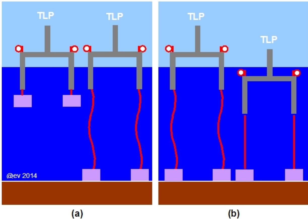
**Figure 83** Schematic diagram of (a) tension-leg platform under tow with seabed anchors held up by cables on left-hand side; platform with seabed anchors lowered and cables lightly tensioned on right-hand side. (b) TLP free floating on left-hand side; structure is pulled by the tensioned cables down towards the seabed anchors) on right-hand side
