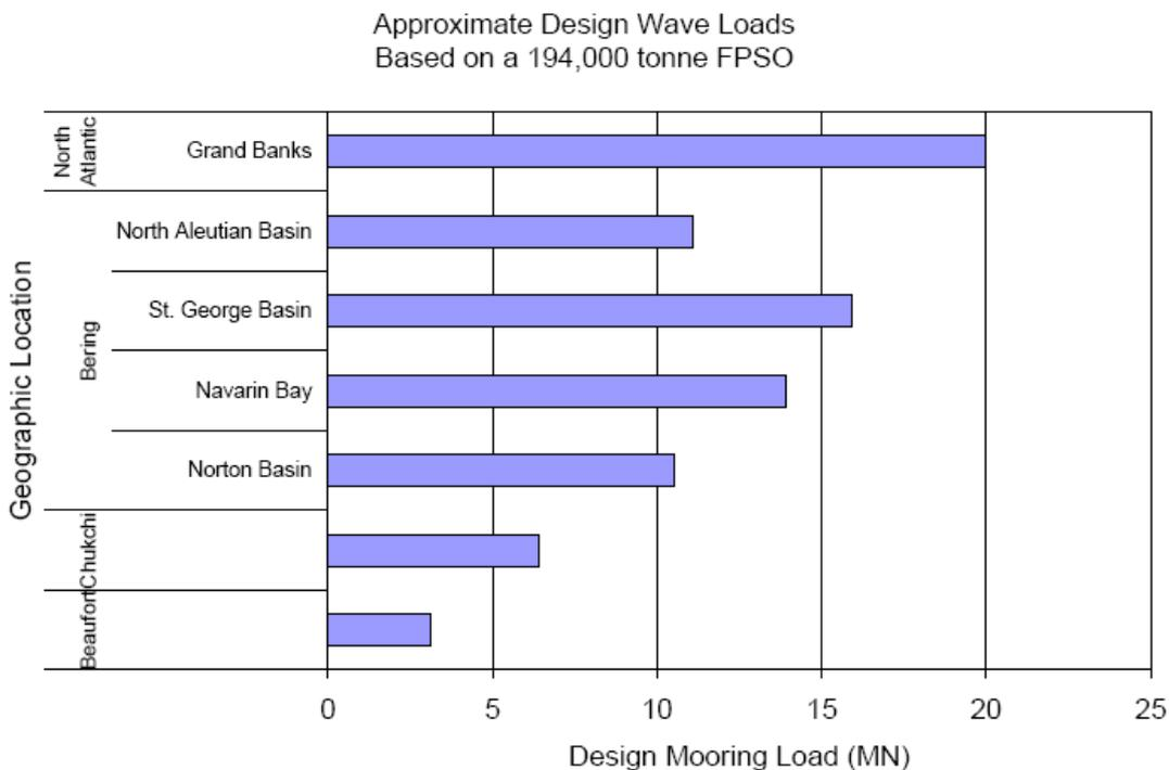
**Figure 101** Approximate design wave loads – FPSO basis (note: wave loads for the Beaufort and Chukchi Sea are for summer conditions and are not meant to imply year round FPSO operations), (IMVPA, 2008)
