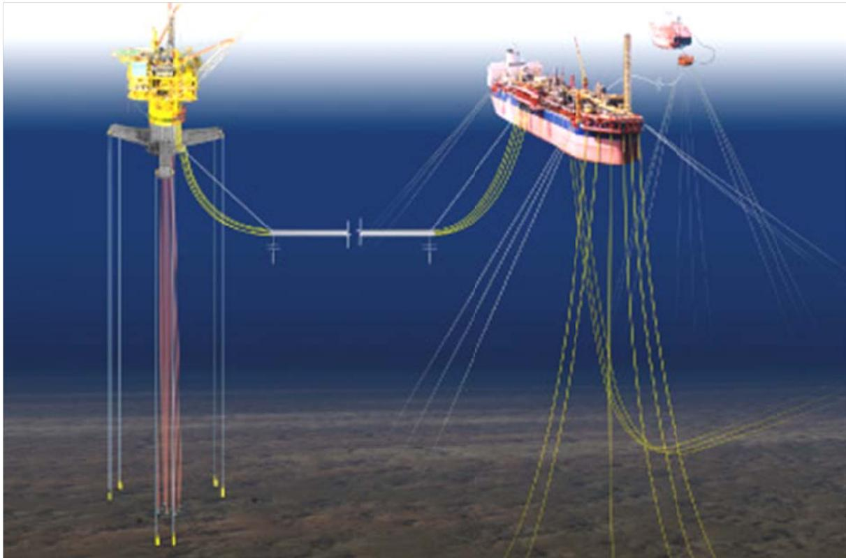
**Figure 82 Illustration of TLP and FPSO with multiple riser<sup>27</sup> configuration**
