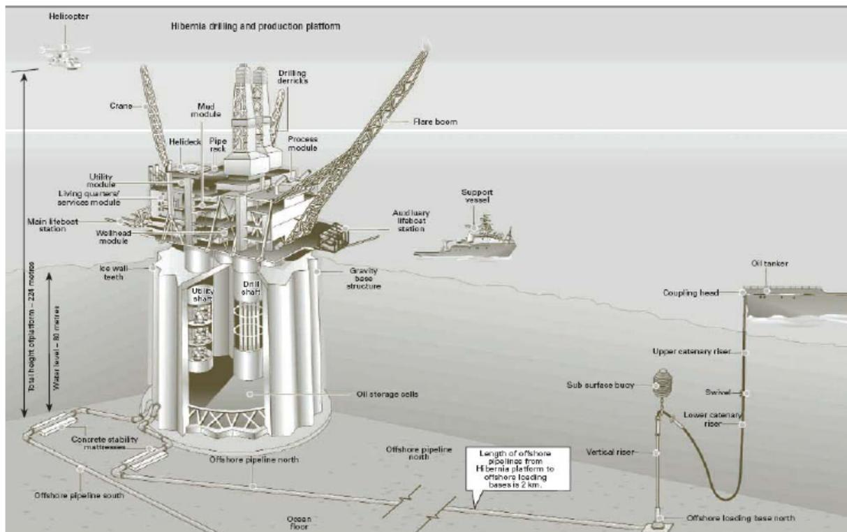
**Figure 27 Hibernia Drilling and Production Platform with Offshore Loading System (OLS), (Bott, 2004)**
