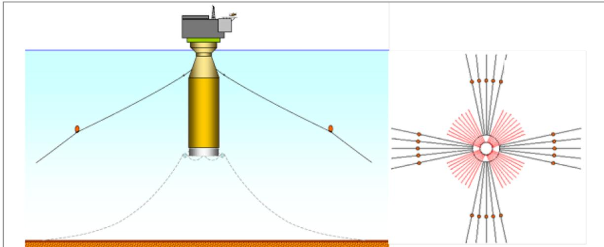
**Figure 92** Vertical plane view of mooring lines (left) and horizontal projection of 20 lines mooring system in 4 groups with 5 lines in each group (right), [Bruun et al. 2009]
