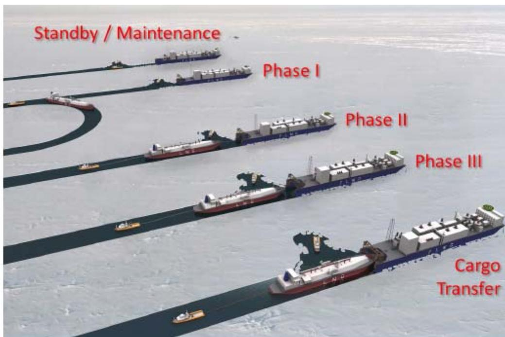
**Figure 62** Steps of approach and pull-in of the carrier to the 'Mooring Bay' and cargo transfer in ice conditions (*Hoog et al., 2012*)
