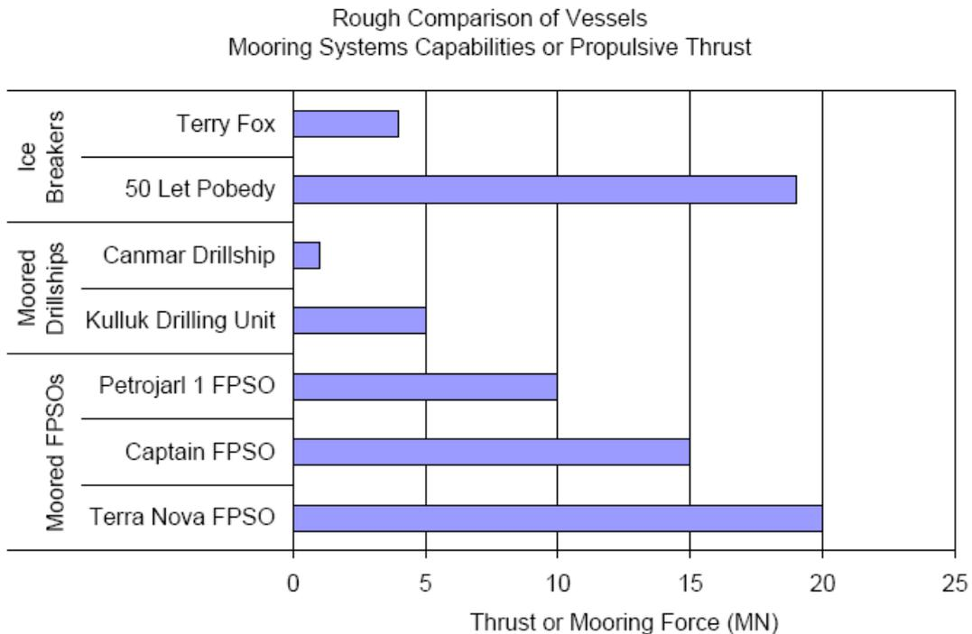
**Figure 103 Comparison of selected vessel mooring systems; with selected icebreaker bollard thrust (*Comfort et al., 2001*)**
