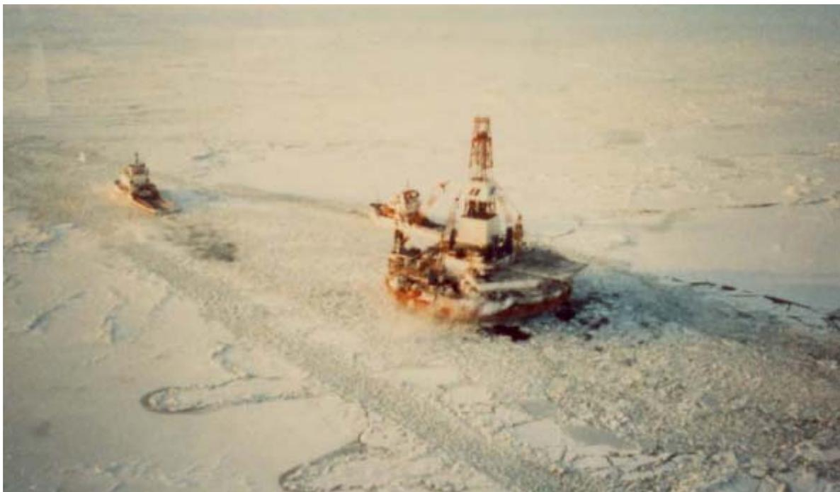
**Figure 74** The Kulluk - Operations with Icebreaker Support (courtesy of *DC Marine*)
