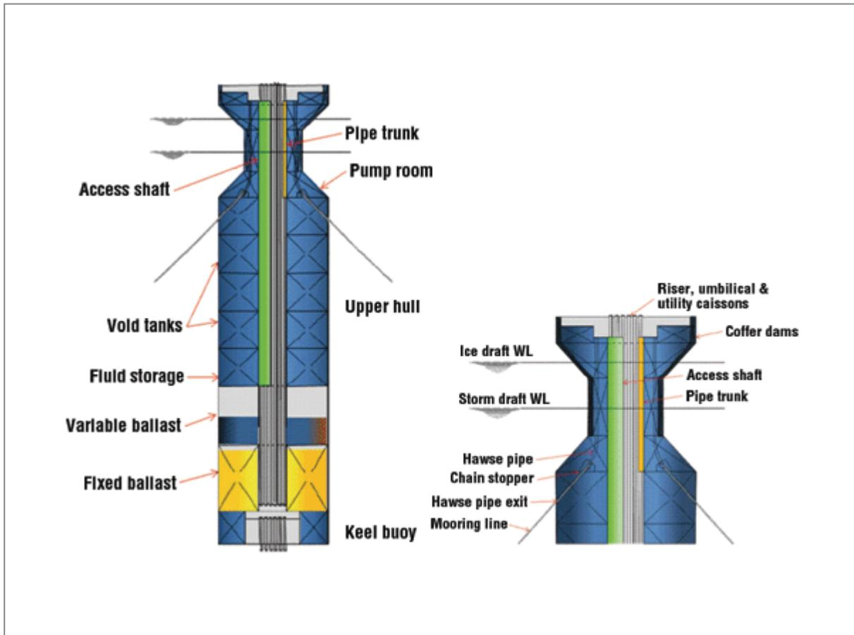
**Figure 95 Schematic diagram of SPAR components (Ghoneim 2011)**
