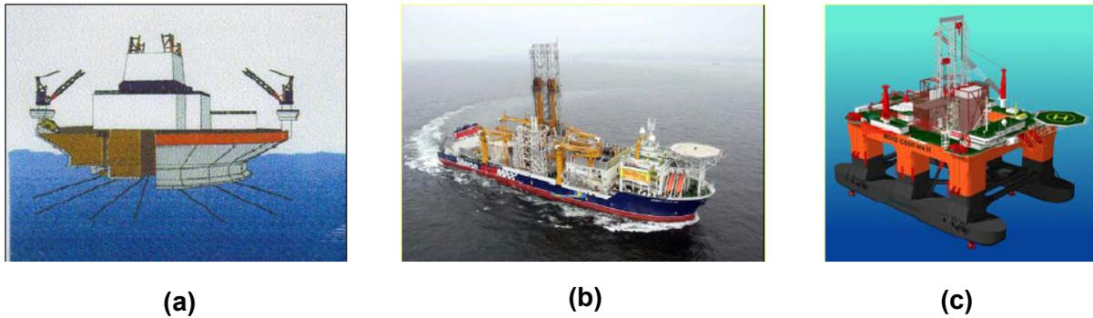
**Figure 65** Floating systems for offshore drilling in the Arctic: (a) drilling rig Kulluk, (b) drillship Stena DrillMax ICE and (c) semi-sub rig designed by Moss Maritime
