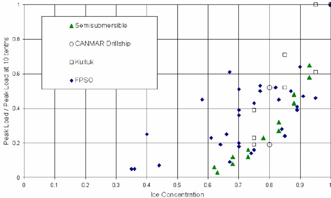
**Figure 100 Peak loads in managed ice – effect of ice concentration on various structure types (reproduced from *Comfort et al., 2001*)**
