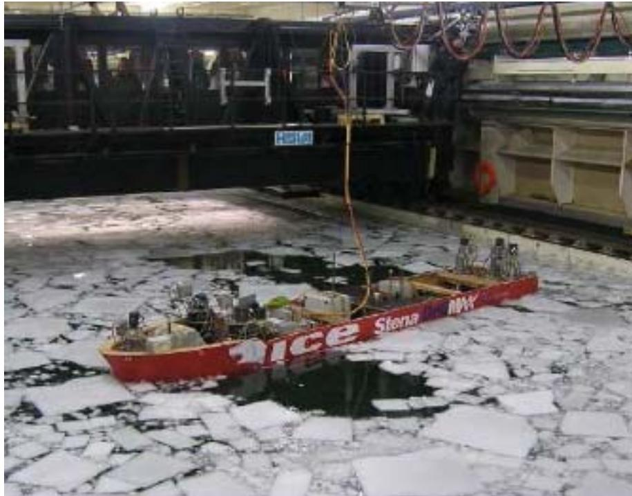
**Figure 77** Ice model tests with Stena DrillMAX ICE model in managed ice
