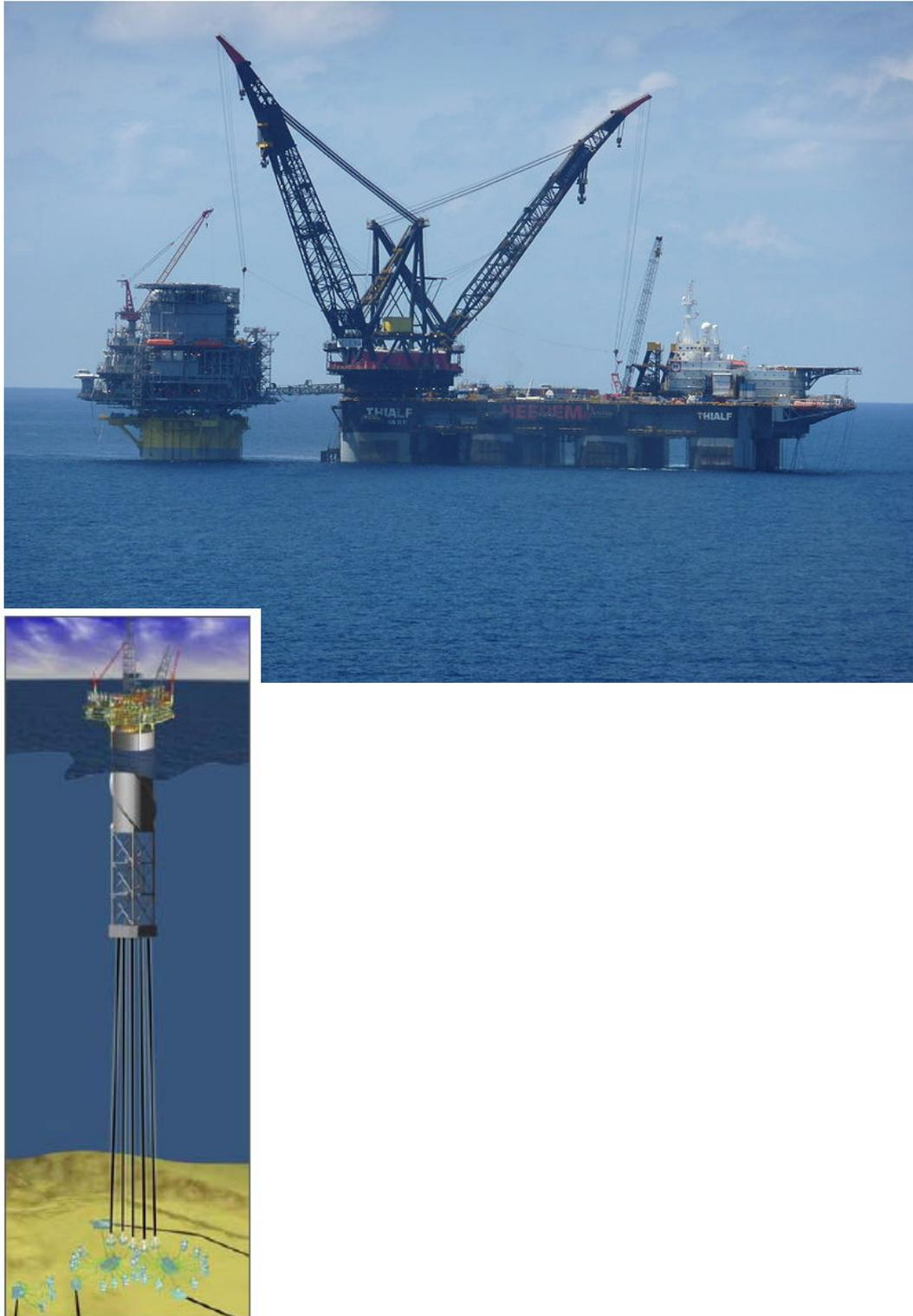
**Figure 96** SPAR platform *Perdido* (left) with SSCV<sup>28</sup> *Thialf* (right) in the Gulf of Mexico in 2450 m waterdepth (source *Wikipedia*)
