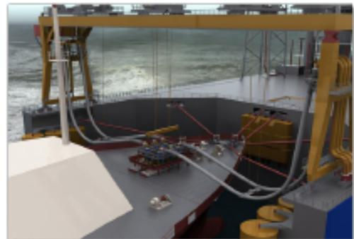
**Figure 61** Safe and reliable handling of the flexible pipes for cargo transfer and in ESD<sup>17</sup> situations (Hoog *et al.*, 2012)
