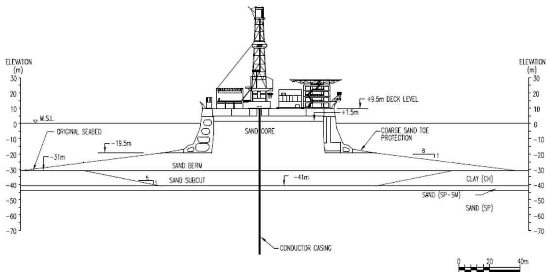
**Figure 8 Cross-section view of the Molikpaq at the Amauligak I-65 site in 1985-1986 (Timco and Johnston, 2002)**
