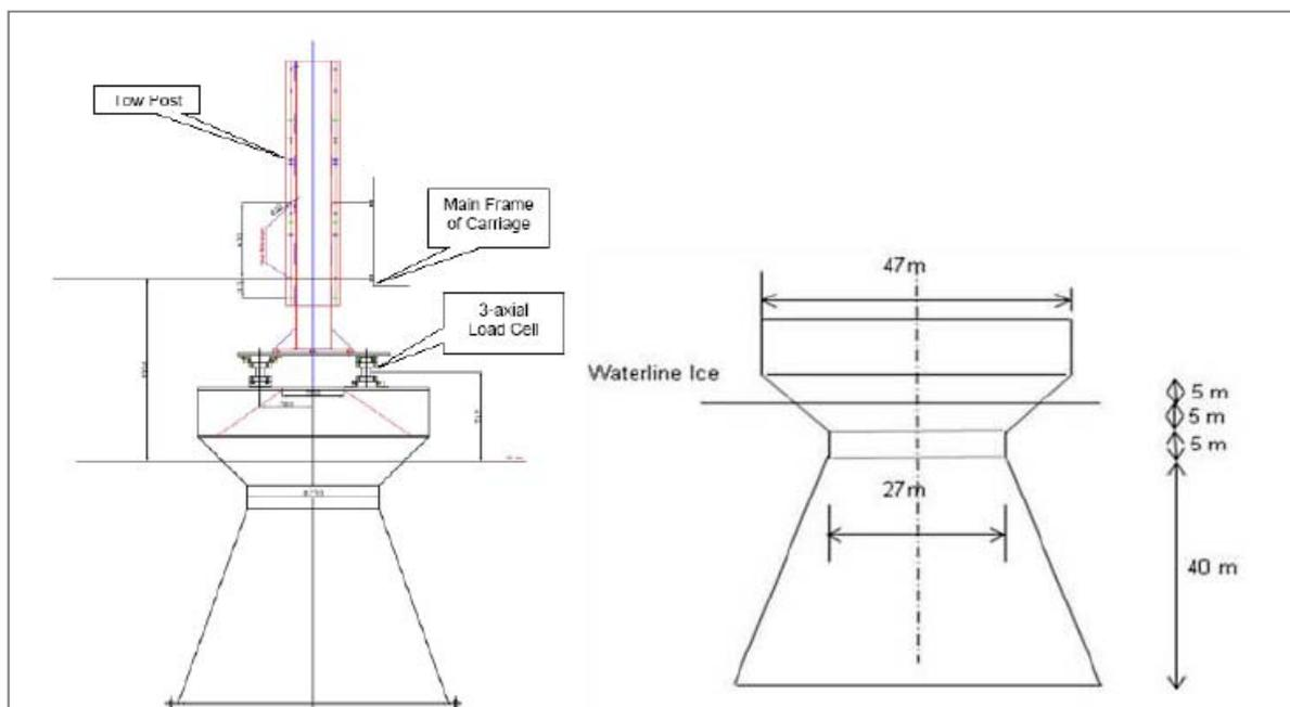
**Figure 91** Fixed model set-up and geometry, representing the upper part of the SPAR (*Bruun et al., 2009*)
