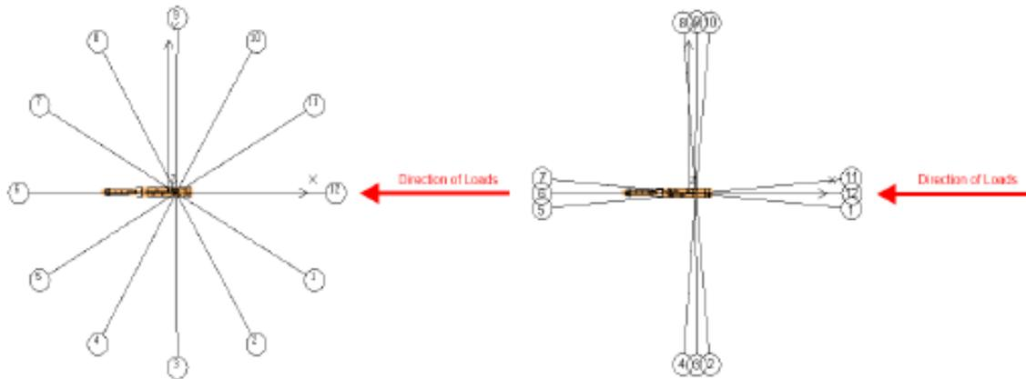
**Figure 63** The analyzed mooring line configurations: 12x1 (left), and 4x3, with angle of attack 180° at each (*Hoog et al., 2012*)
