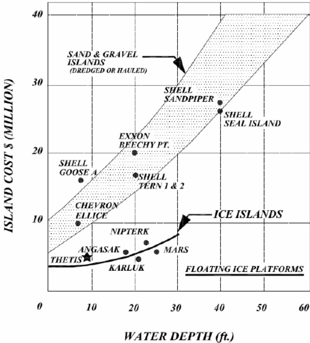
Figure 21 Cost comparison between gravel and ice islands (C-CORE, 2005)
