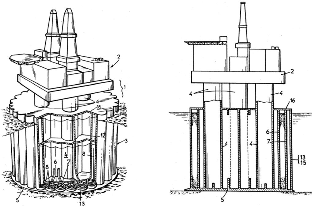
**Figure 30** Monolithic concrete caisson for Arctic regions (US Patent 5044830 A)
