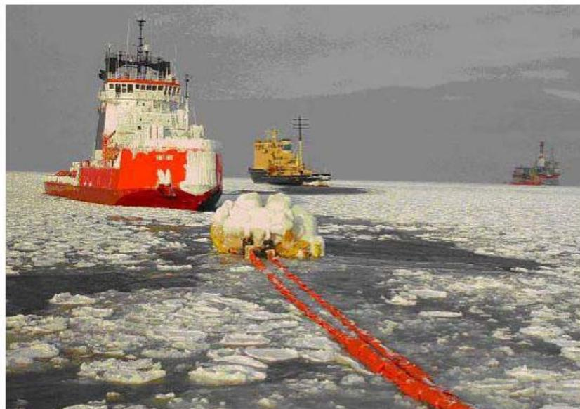
**Figure 97 Icebreaker „Smit Sibu“ providing ice management operations for SALM buoy lay down operations on Sakhalin (courtesy of Don Conelly)**
