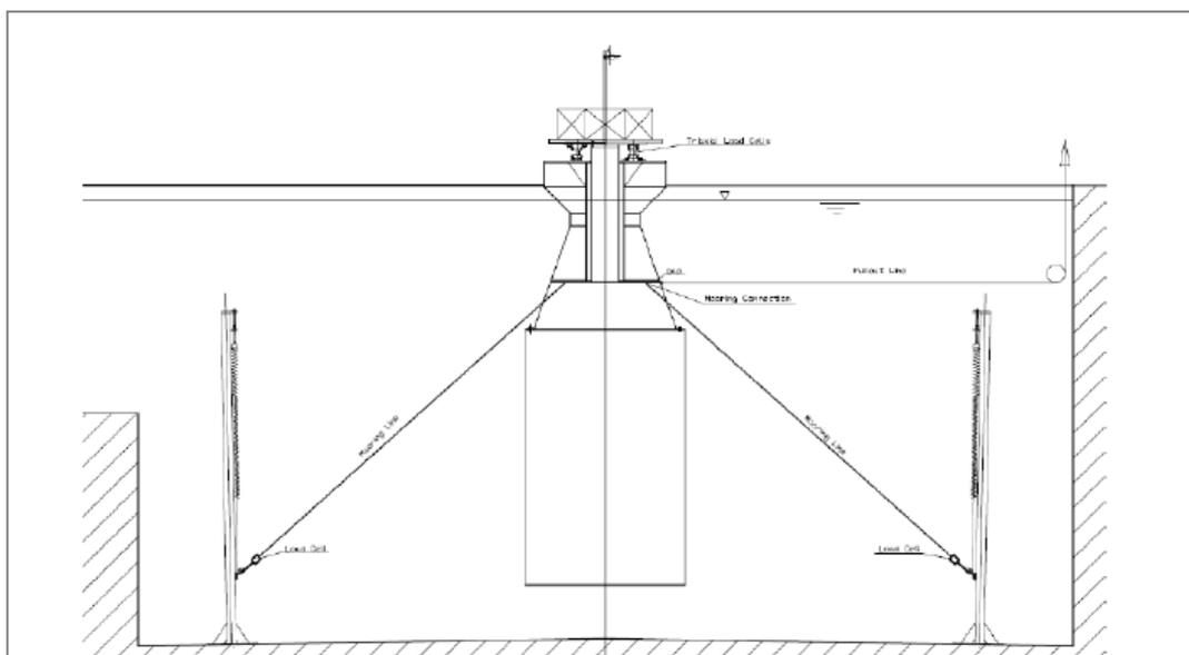
**Figure 93** Schematic diagram of mooring system (Bruun et al., 2009)
