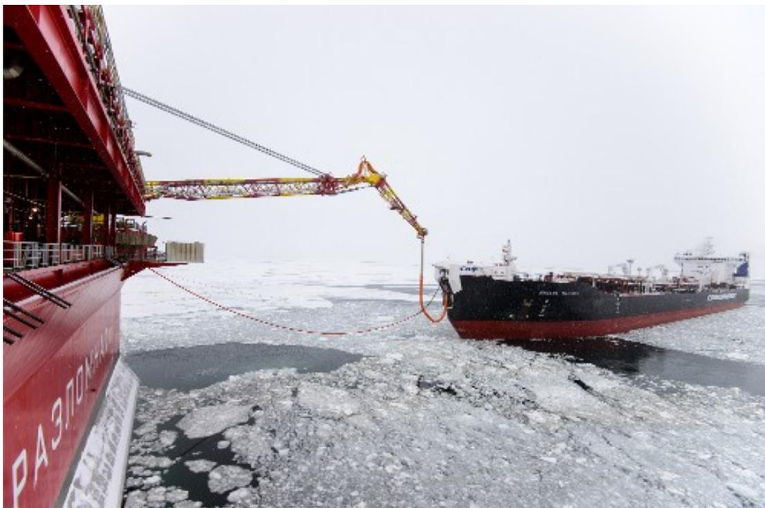
**Figure 46** Oil transfer from production platform to icebreaking shuttle tanker MT “Mikhail Ulyanov” (source: *Gazprom*)
