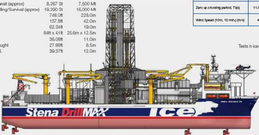
**Figure 76 Drillship Stena Drill MAX ICE (courtesy Stena)**
