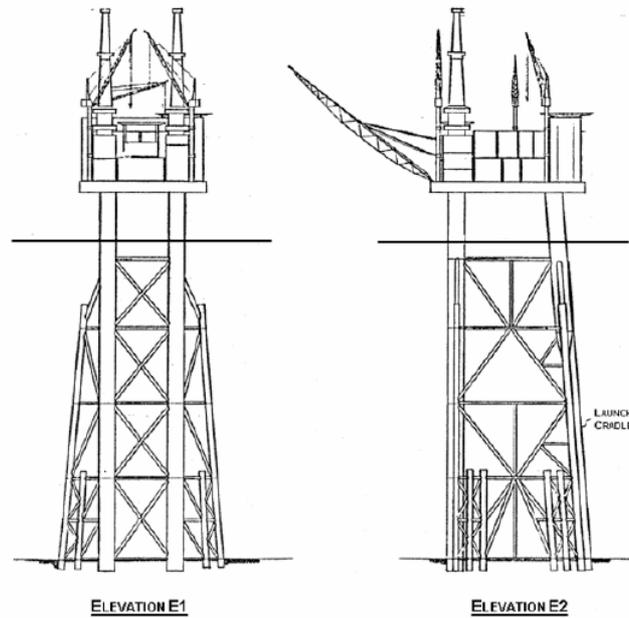
**Figure 22** Four plus Four Template Jacket (modified from *PMB Systems Engineering et al., 1983*)
