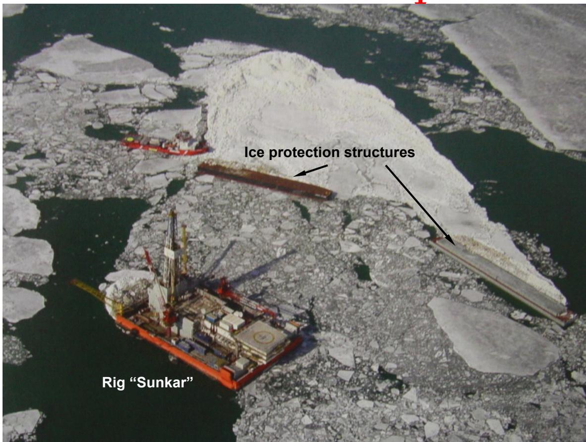
**Figure 37** Drilling rig “Sunkar” surrounded by ice protection structures (grounded steel barges)
