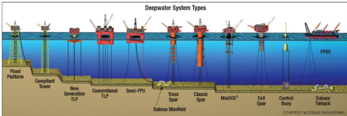
**Figure 67 Deepwater system types (source: Mustang Engineering)**
