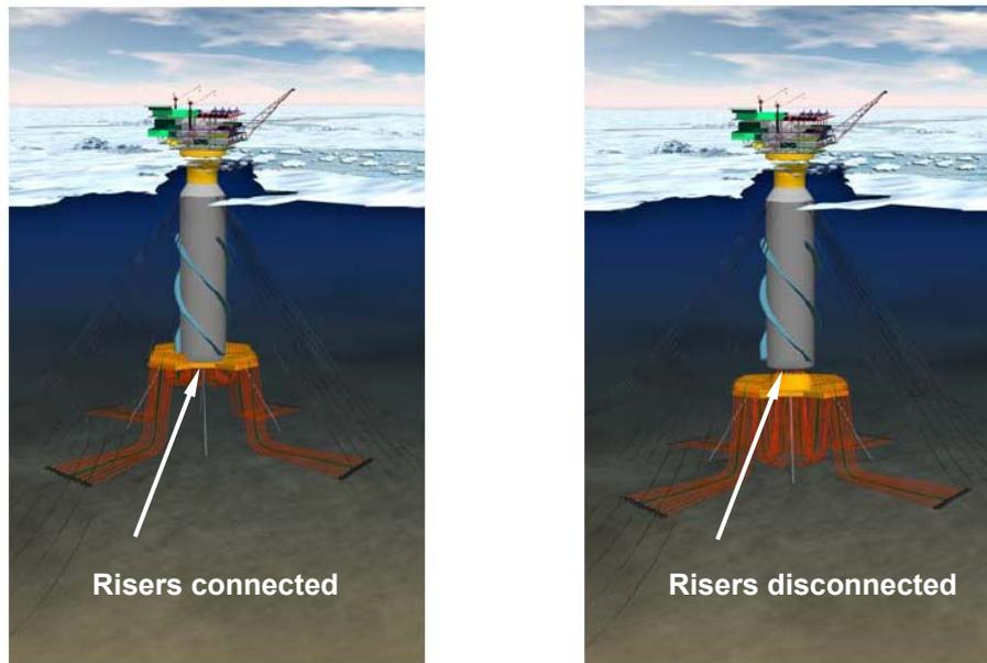
**Figure 94** Artist's cut-away of the Arctic Spar with risers connected (left) and disconnected (right), (after Ghoneim, 2011)
