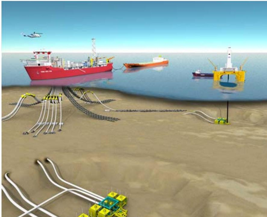
**Figure 70 Illustration of pathway for oil and fluids that flow to and from the FPSO and reservoir (source: Suncor)**
