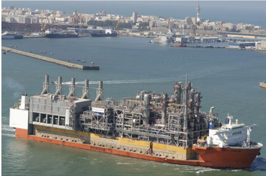
**Figure 57** Dragados Offshore began construction of the 33,000-ton processing plant producing liquefied natural gas in June 2003. On 13 July 2005, the system was put in place in the dock at Melkøya outside Hammerfest (source: Statoil).
