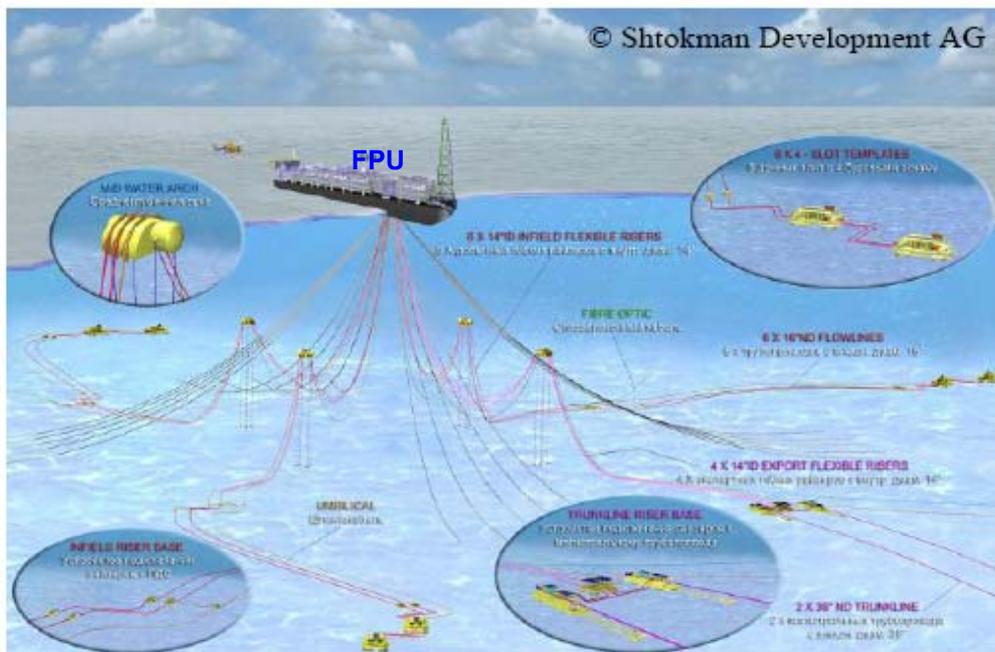
**Figure 47 Schematic scheme of offshore installations of the Shtokman project (*Bambulyak and Frantzen, 2011*)**
