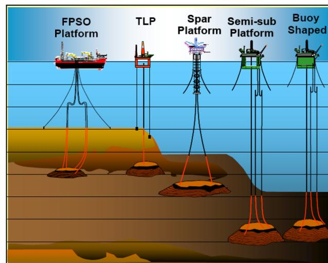
**Figure 66** Alternative floating platform designs in deepwater
