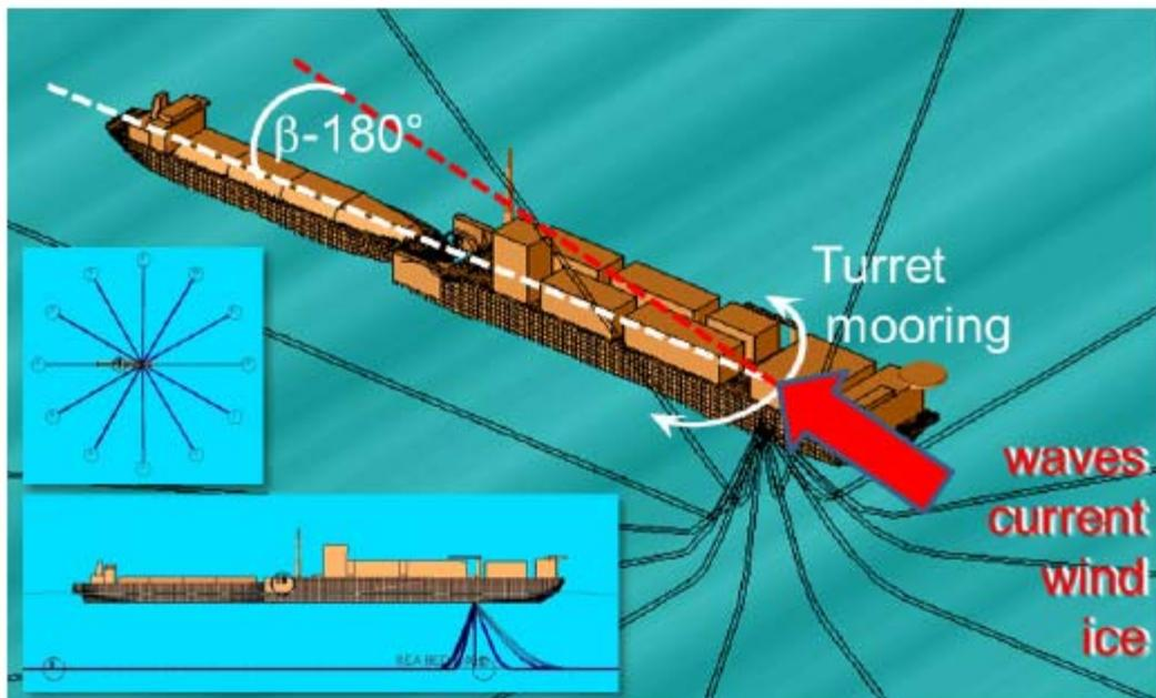
**Figure 59** The turret mooring concept allows weathervaning as response to changing load directions (*Hoog et al., 2012*)
