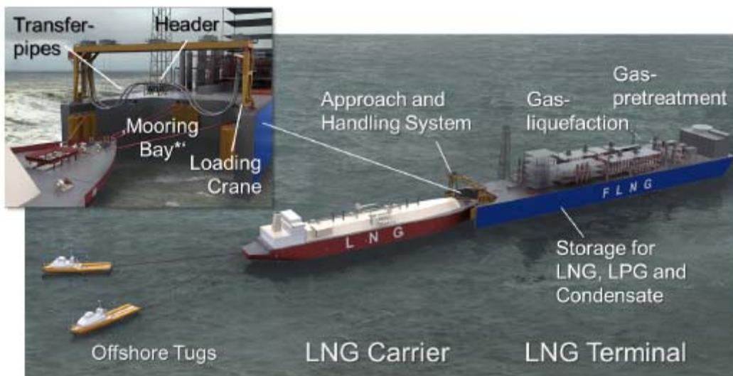
**Figure 60 Main components of the MPLS20 concept (*Hoog et al., 2012*)**
