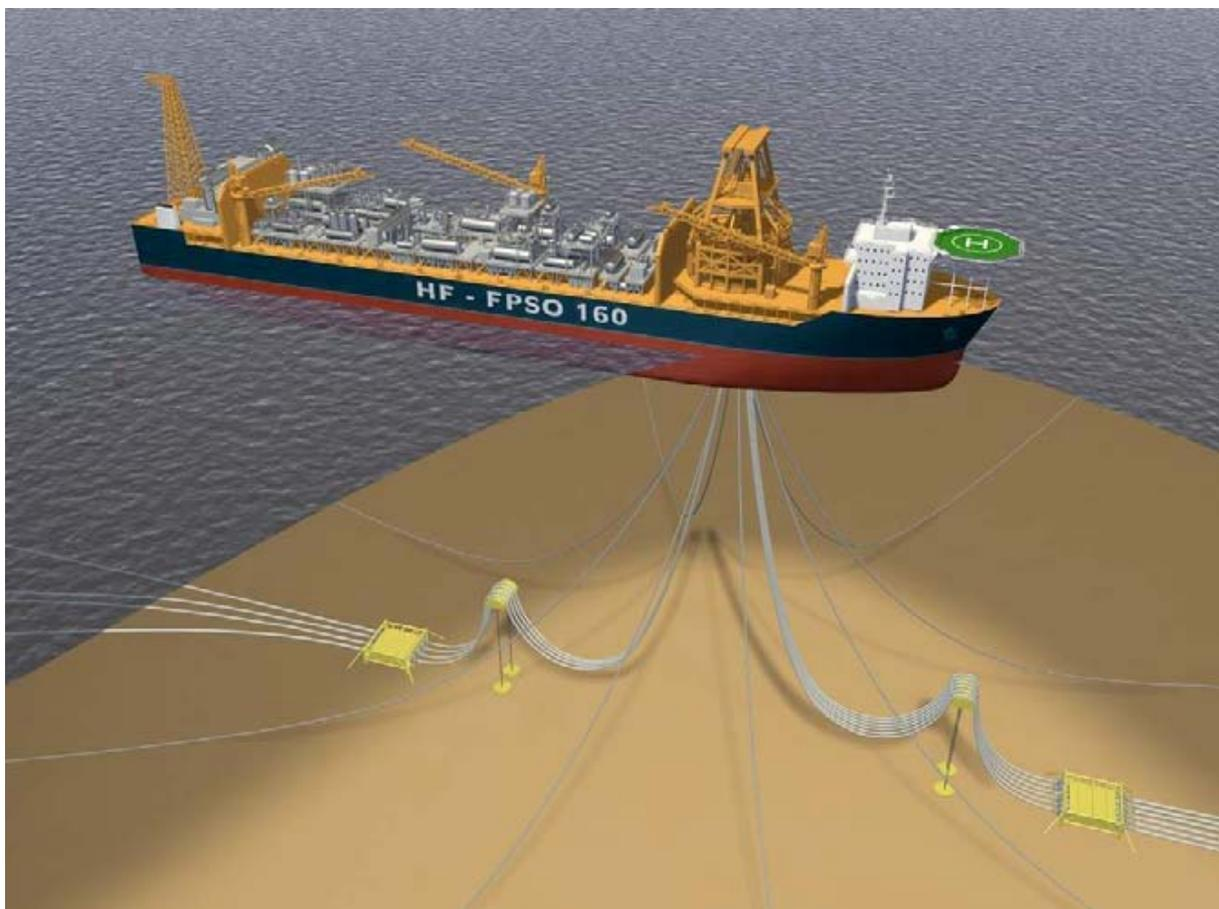
**Figure 81** Illustration of Floating Production Storage and Offloading (FPSO) with flowlines and risers (source: [corrosion-doctors.org](http://corrosion-doctors.org))
