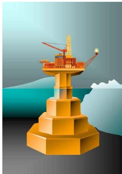
**Figure 29 Steel Stepped Gravity Base Structure**
