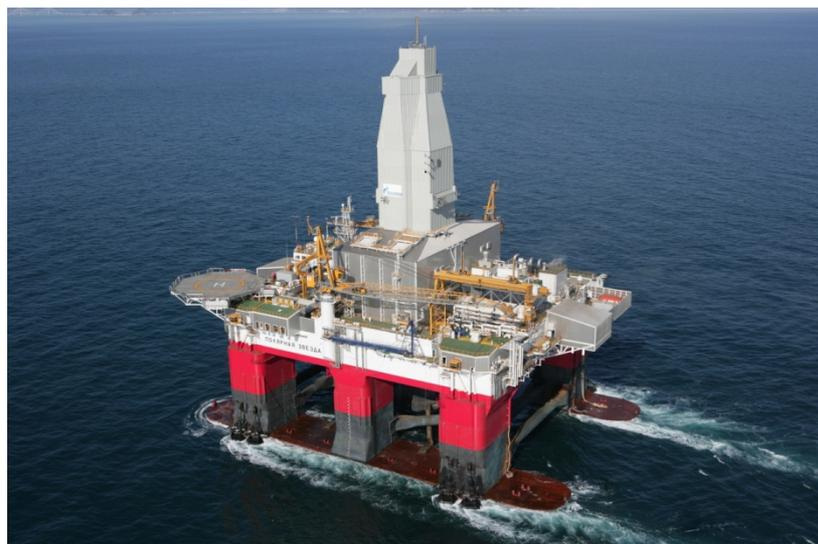
**Figure 80** Semi-submersible floating drilling rig Polyarnaya Zvezda (Polar Star) drilling in Kirinskoye field (Sakhalin III Project), [source: *Gazprom*]
