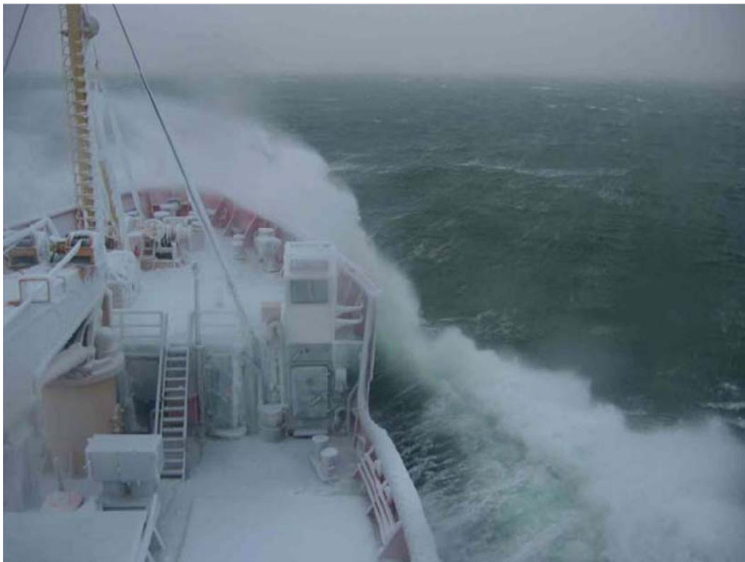
Figure 28 Severe icing conditions (source: Canadian Coast Guard )
