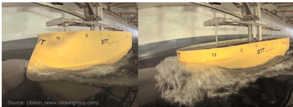
Figure 25 Spray generation of different bow types: Ulstein X-Bow® ( left ) compared to a conventional formed bow ( right )
