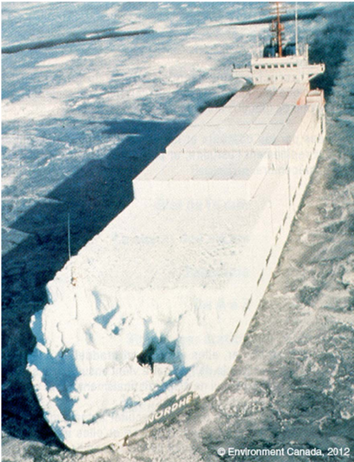
Figure 32 Sea spray icing on a container vessel (source: Canadian Coast Guard )
