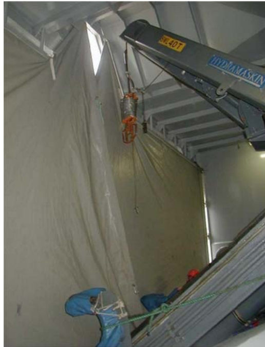
Figure 39 Tarpaulin installed to protect cranes or rescue boats ( Koren, 2007 )
