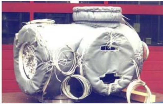
Figure 42 Heating jacket and heating cable for moveable parts and pipes ( ClassNK, 2009 )
