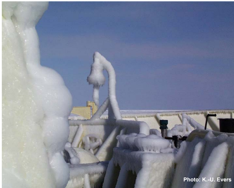
Figure 31 Severe ice build-up on the forecastle of Russian icebreaker “ Kapitan Dranitsyn ” during voyage in Ob Bay (Russia)
