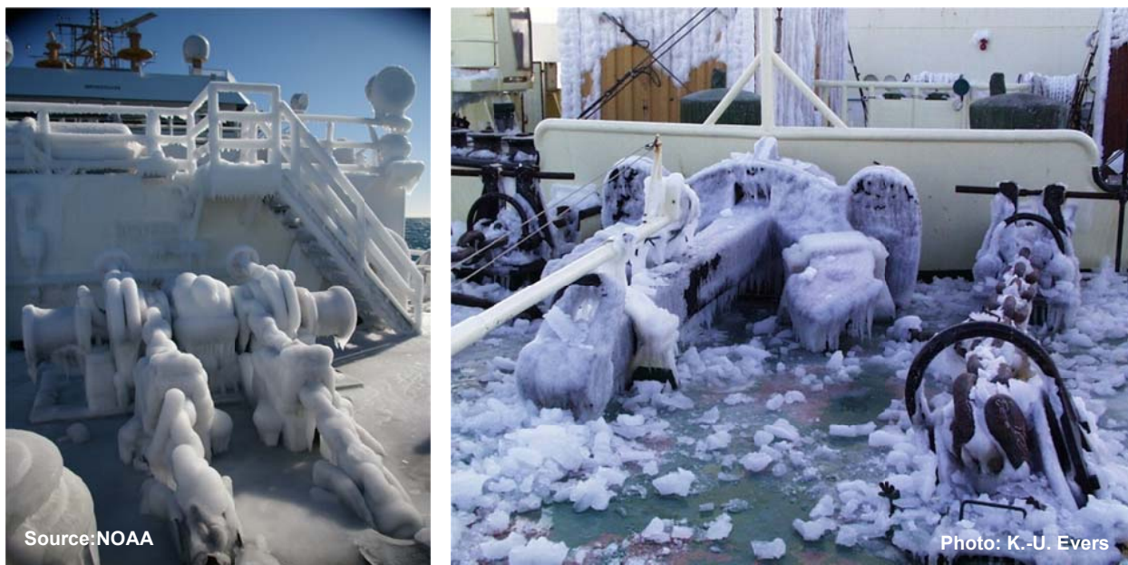
Figure 33 Icing on anchor windlass on board of NOAA ship “ Oscar Dyson ” (left) and Russian icebreaker “ Kapitan Dranitsyn ” (right).
