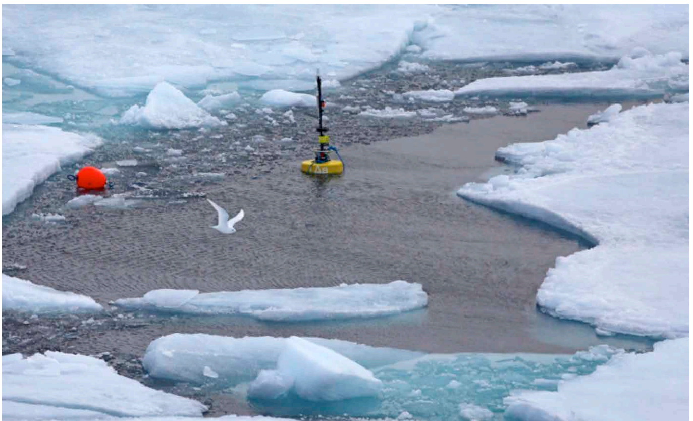
Figure 5 - Deployment of Passive Acoustic Sensors in Northeast Greenland (ODEN Arctic Technology and Research Cruise 2013). Photo: Jan Durinck.
