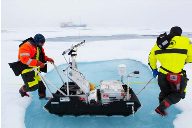
Figure 12 - Scientists from NPI measuring radiative energy balance of ponded sea-ice using the "radiation sled." Courtesy of Tor Ivan Karlsen (Norwegian Polar Institute)
