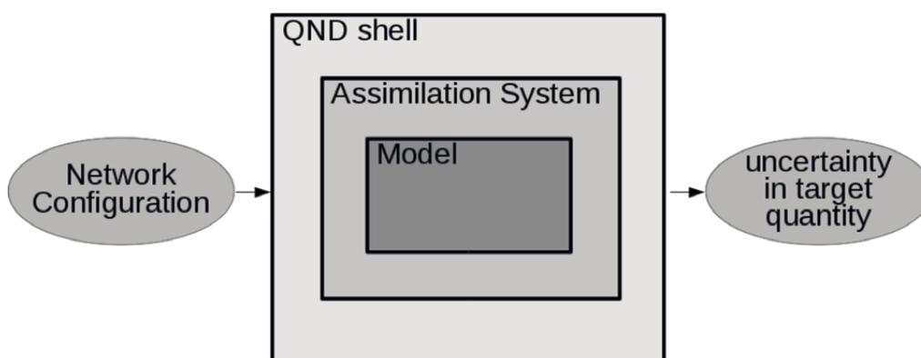
Figure 5 - Schematic Presentation of Quantitative Network Design Procedure. Network configuration includes samples quantities, sampling times and locations and data uncertainty.
