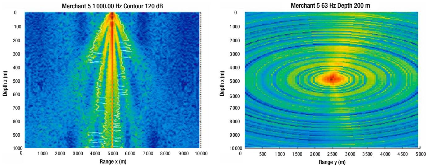
Figure 17 - Screen shots of the directivity noise pattern at different ranges from a merchant ship from the simulator at (left) 1000 Hz and (right) 63 Hz at a depth of 200 m.
