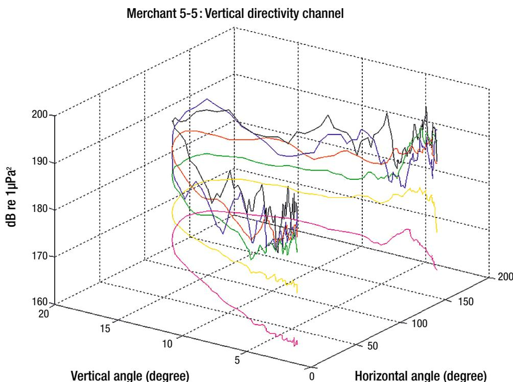
Figure 16 - Noise directivity diagram from a merchant vessel in vertical and horizontal degrees.
