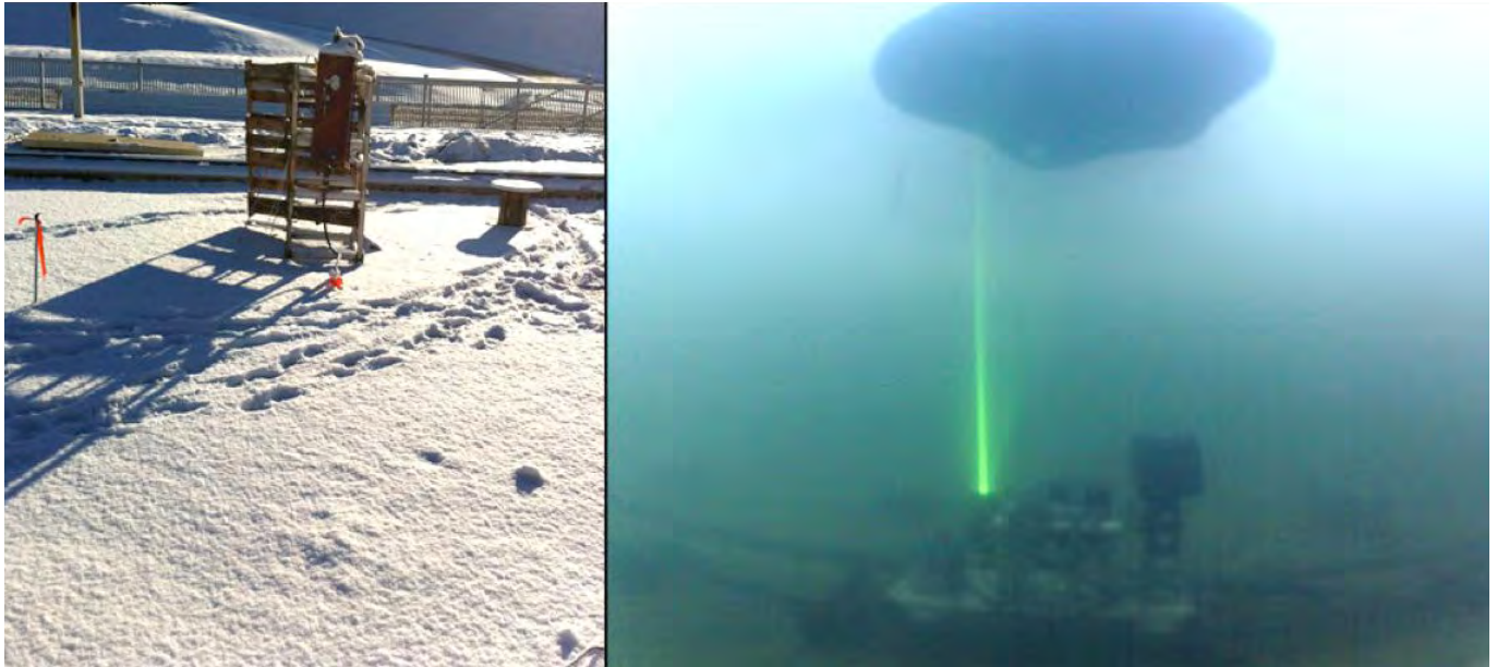
Figure 12: Oil spill experiments at the United States Army Cold Regions Research and Engineering Laboratory in Hanover, USA. Oil was injected under the ice from above (left), and a suite of instruments, including cameras, sonar, and a laser system, were placed on a trolley beneath the slick (right). This work was partly funded by the Oil Spill Recovery Institute ( http://www.pws-osri.org/ ). With permission Jeremy Wilkinson.
