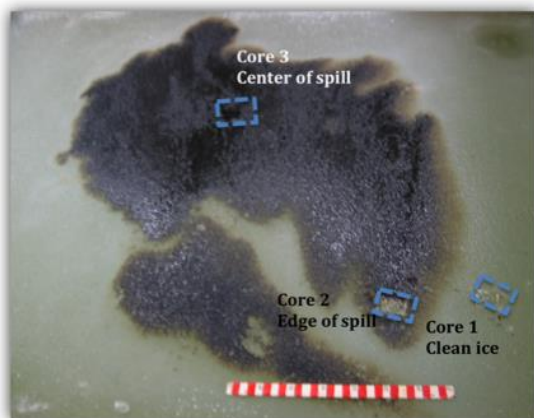
Figure 18. Results of the simulated spill in frazil ice. Most of the oil spread across the surface of the frazil. The blue boxes indicate where cores were taken and frozen for further analysis.
