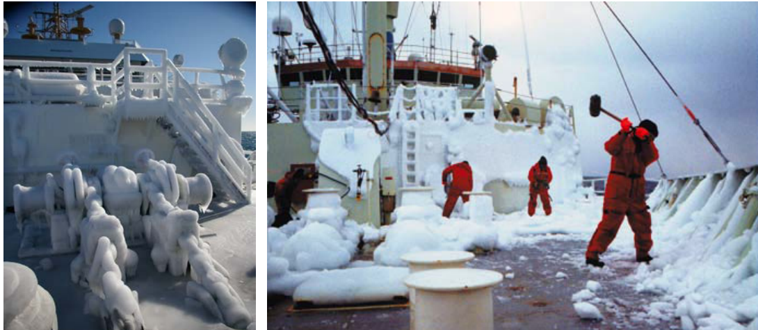
Figure 8-1: Ice built-up and manual de-icing of a ship's deck
