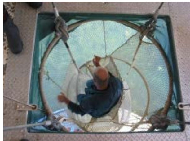
Figure 8-8: Evacuation from offshore platforms via fall net for single persons and liferafts
