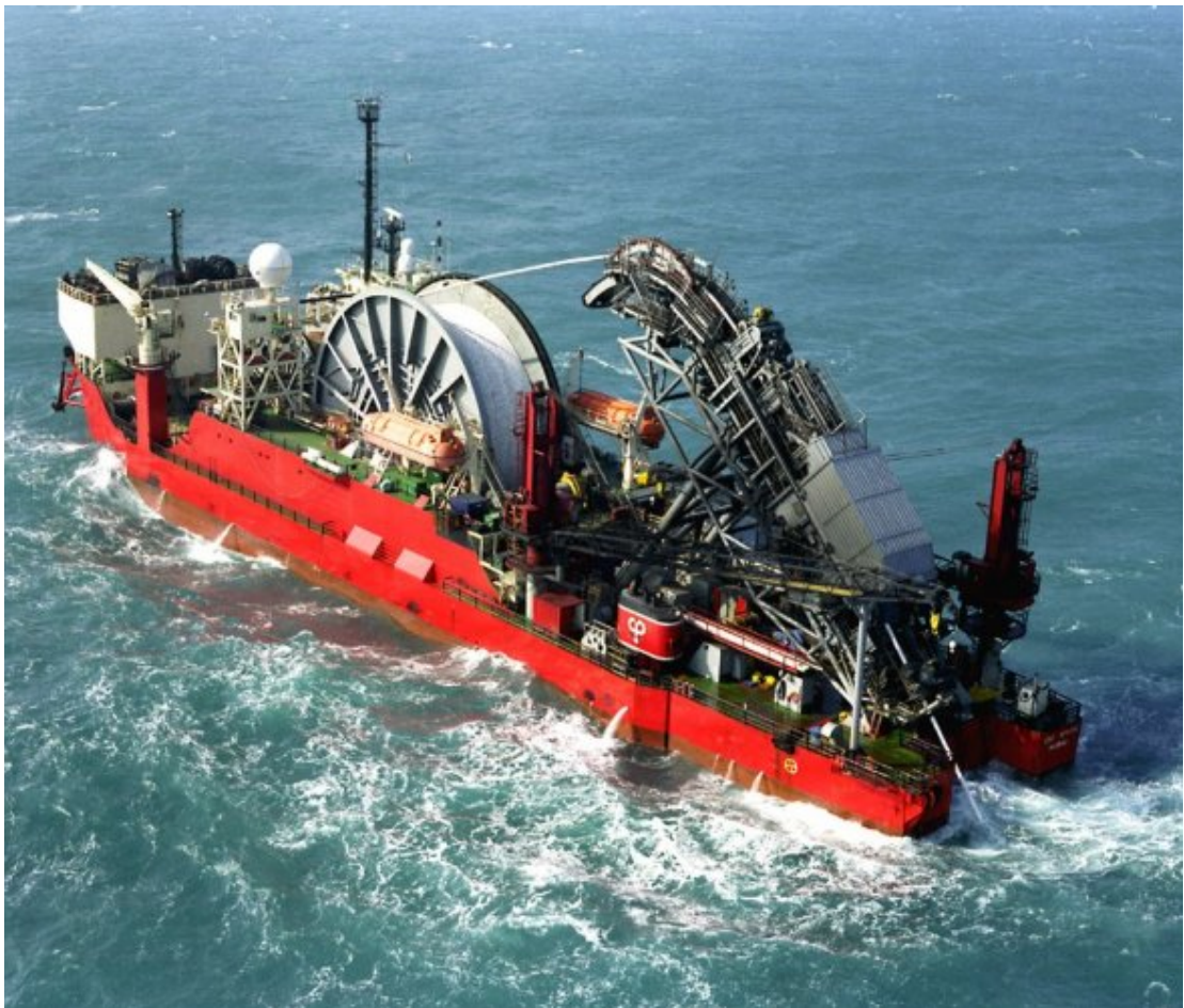
Figure 11-19: Cable lay vessel with dynamic positioning (DP)
