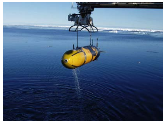
Figure 11-15: ROV at an XTree (left, Oceaneering) and AUV during launch for under ice survey (Autosub)
