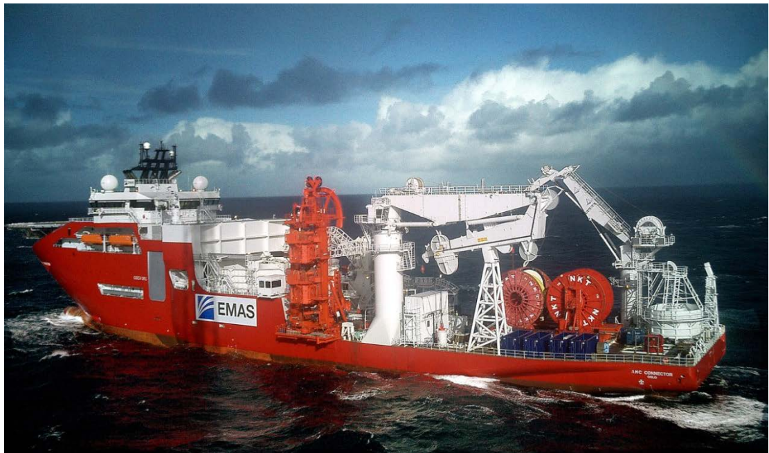
Figure 11-11: Multipurpose construction vessel with crane load capacity up to 300 t
