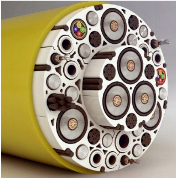
Figure 11-18: Multipurpose subsea umbilical allowing transferring power, data and fluids over long distances
