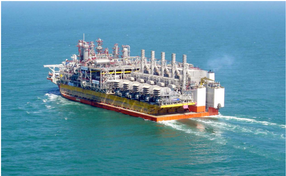
Figure 11-6: Travel of the barge with the Coldbox LNG plant technology on top of a heavy load carrier vessel to Melkøya Island (Linde, Germany)
