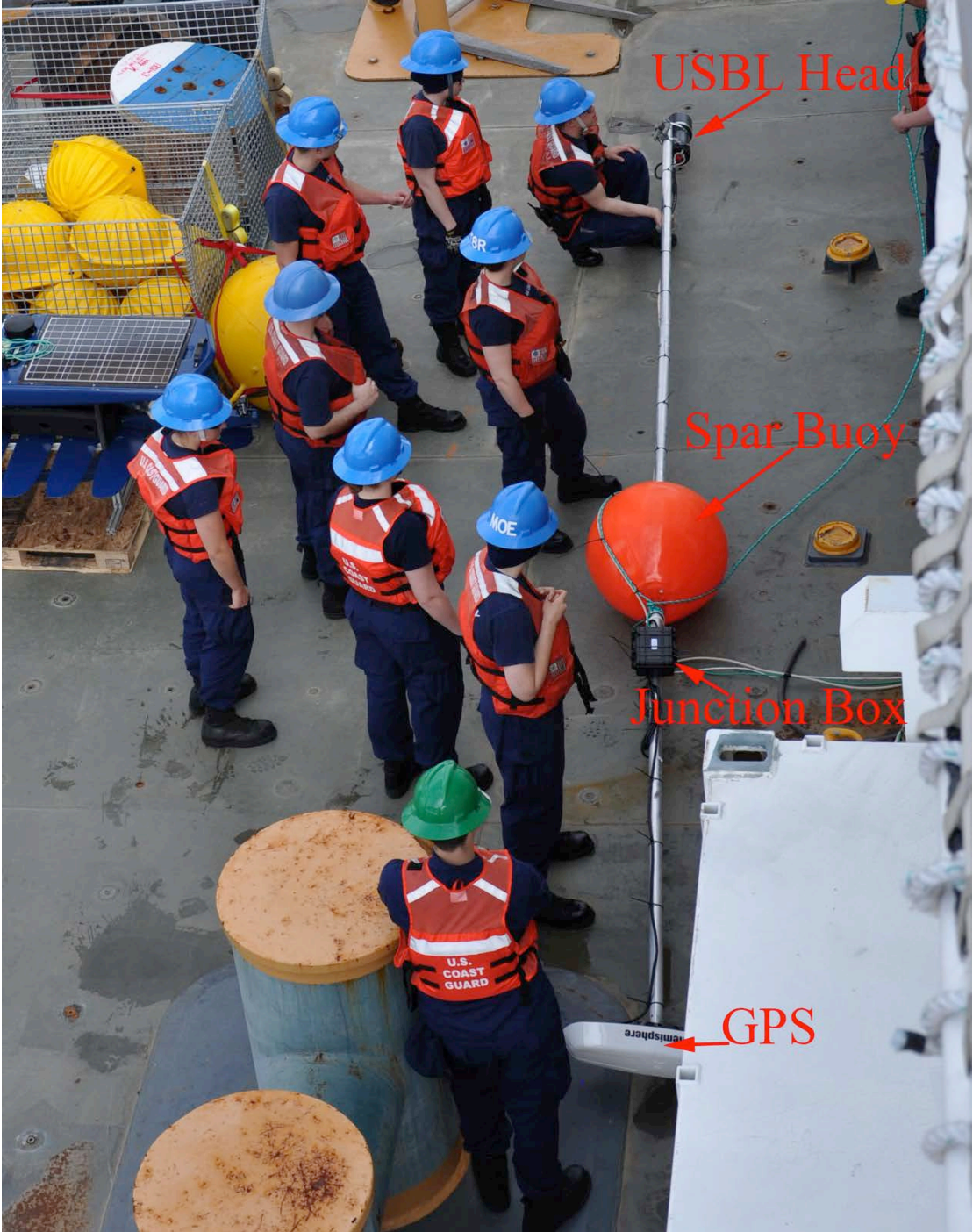
Figure 3.1. Photograph of the tracking buoy, ready for deployment. Two people are necessary for this task.
