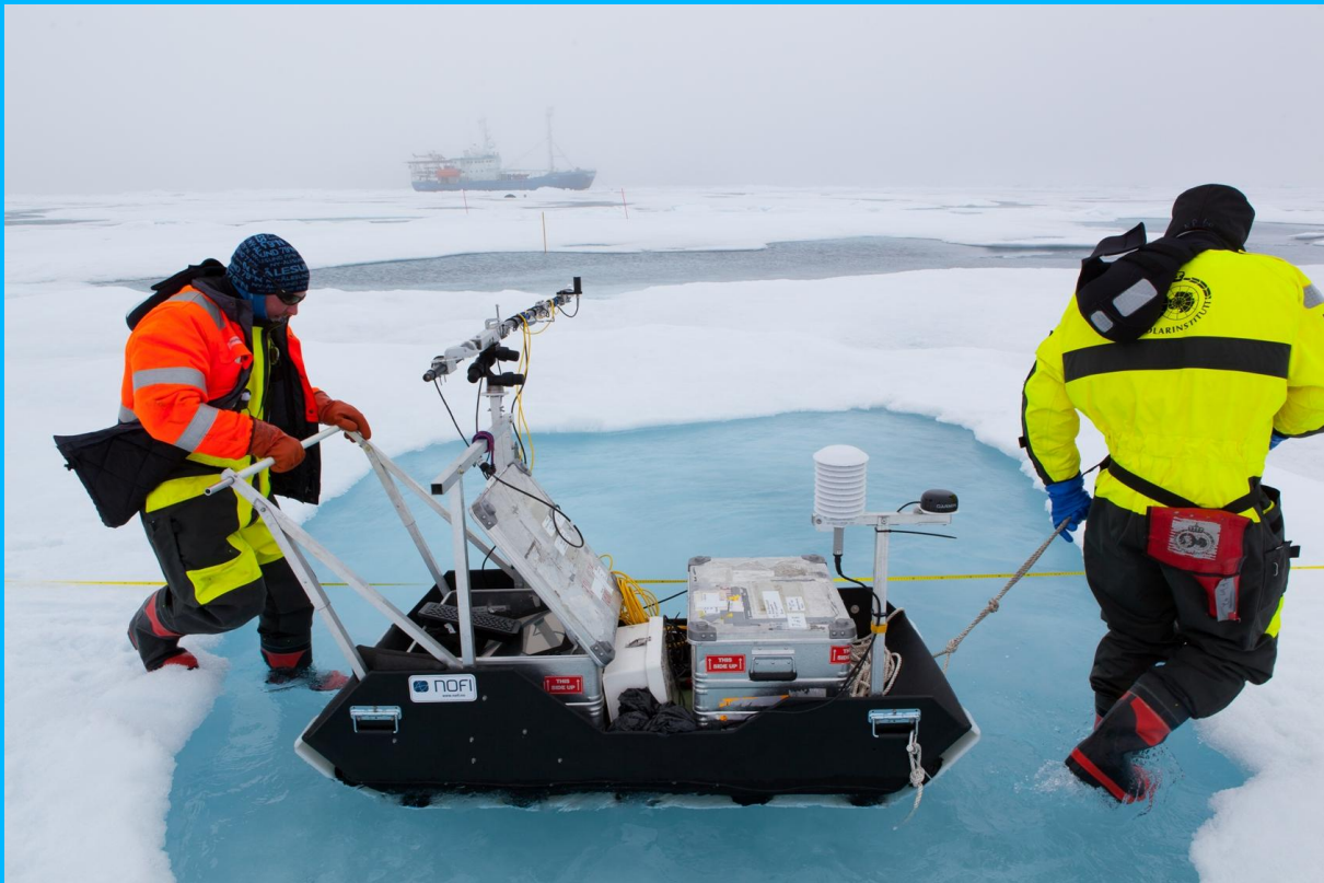
Figure 1 Measuring the optical properties of a melt pond using the radiation sled. Photo: Tor Ivan Karlsen (NPI).
