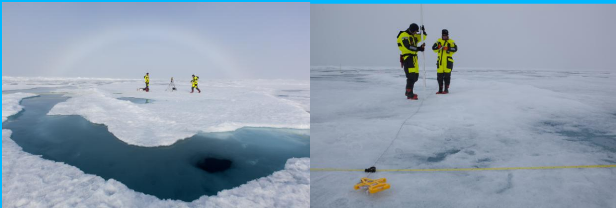
Figure 5 showing measuring the sea ice topography using rotary laser system (image courtesy Tor Ivan Karlsen, NPI).
