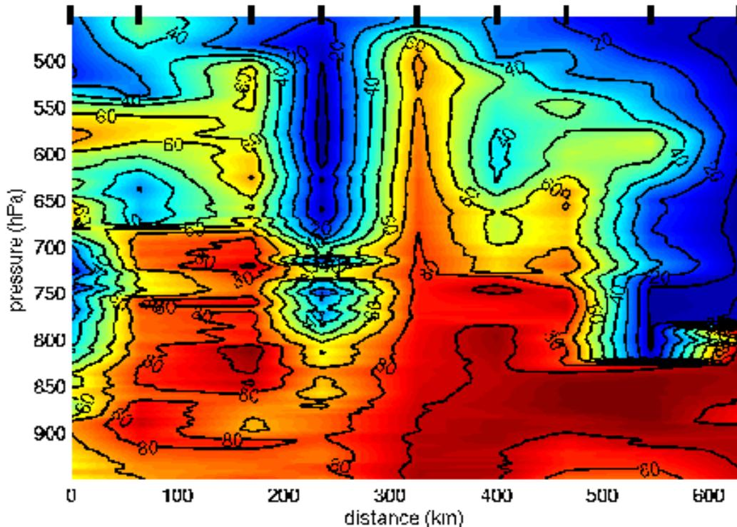
Figure 10: Relative humidity along a section through the polar low observed on 4 March 2008 during the IPY-THORPEX observation campaign. The plot is based on 9 air-craft dropsondes (marked by the black bars on top of the plot) along a straight line the made a slice through the centre of the low. The dry air seen at about 250 km is the eye of the low and is probably caused by intrusion of stratospheric air.
