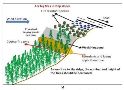
Figure 62. Planting structure to hinder fires in a) flat and b) sloping areas
