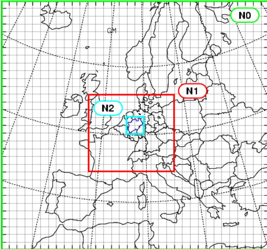
Figure 1: Model configuration from the European scale to the local scale, grid sizes 125, 25, 5, and 1 km. The N1-domain with a grid size for 25 km has been selected für the budget studies in the BeNeLux area.
