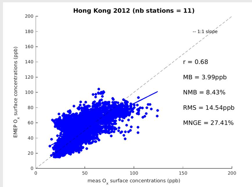
Overestimation in  $O_3$  → clear link with the titration of  $O_3$
